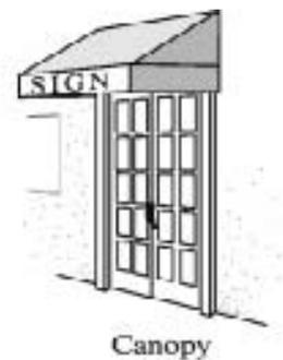
**Canopy Sign:** A building sign that is part of or attached to a canopy, made of fabric, plastic, or structural protective cover over a door or entrance. A canopy sign is not a marquee.
